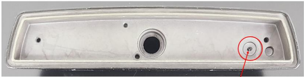
Breather target opening. Secondary drilling operation to create a path into the mounting screw hole so that light can breathe. This hole was filled with silicone to plug until new housings without the drilled hole we available
