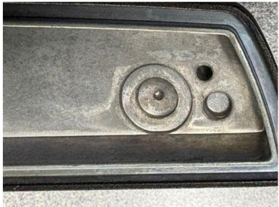
Breather target opening. Secondary drilling operation to create a path into the mounting screw hole so that light can breathe. This hole was filled with silicone to plug until new housings without the drilled hole we available
