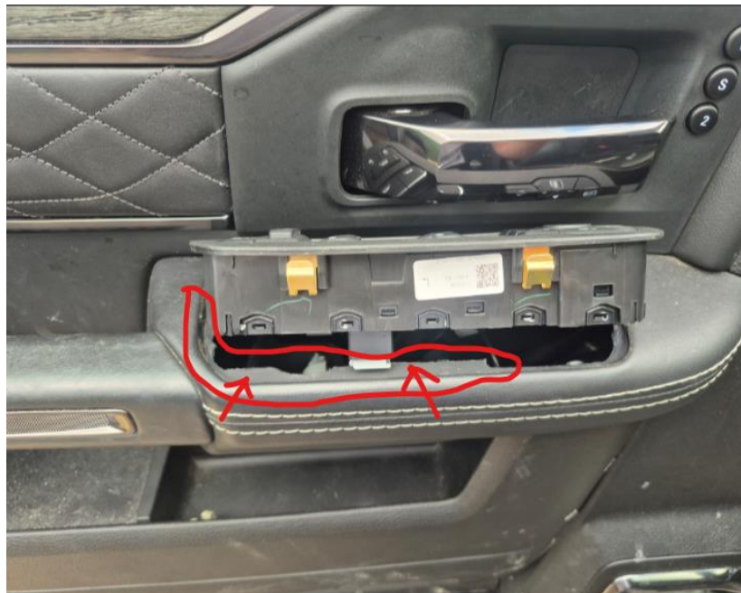
Example Of Excess Material To Be Trimmed. Condition 2
