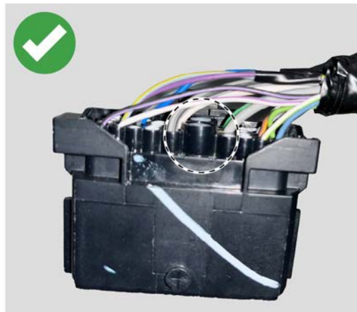
Cavity Plug Properly Seated
