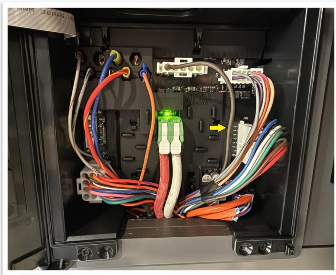
Fig. 2 – 14-gauge brown wire at the 5-pin connector — cut location indicated by arrow.
