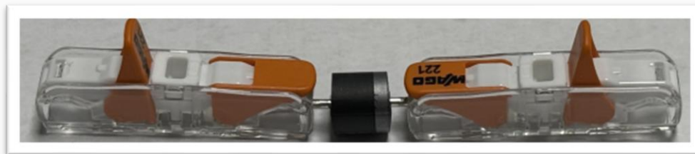
Fig. 3 — Supplied diode with Wago connector — locking levers open.
