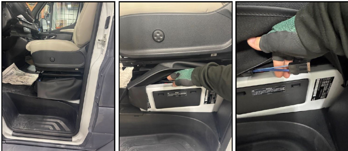
Fig. 1-3 — Location of the 5A fuse
