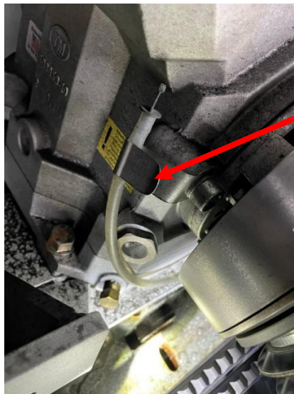
Figure 3: Original location of the oil collection tube
