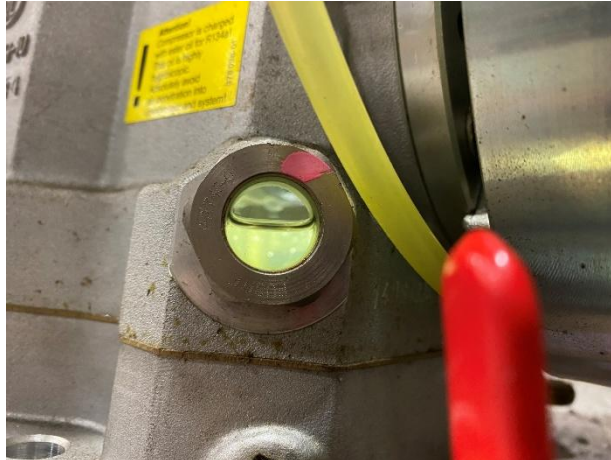
Figure 15: Check oil level
