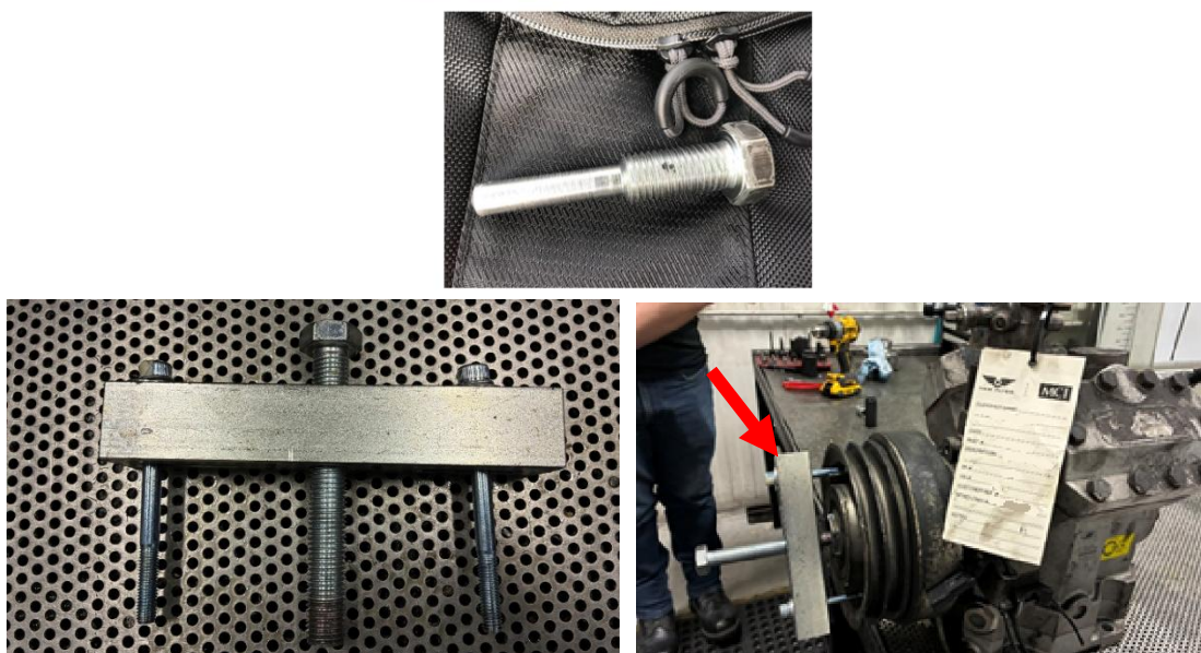
Figure 13: 3-bolt type puller as a second option to remove clutch-pulley assembly
