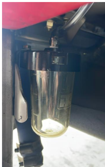
Figure 10: Install bottle and hose
