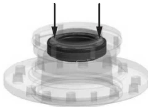
Fig. 1 Sealing cover with stationary ring
