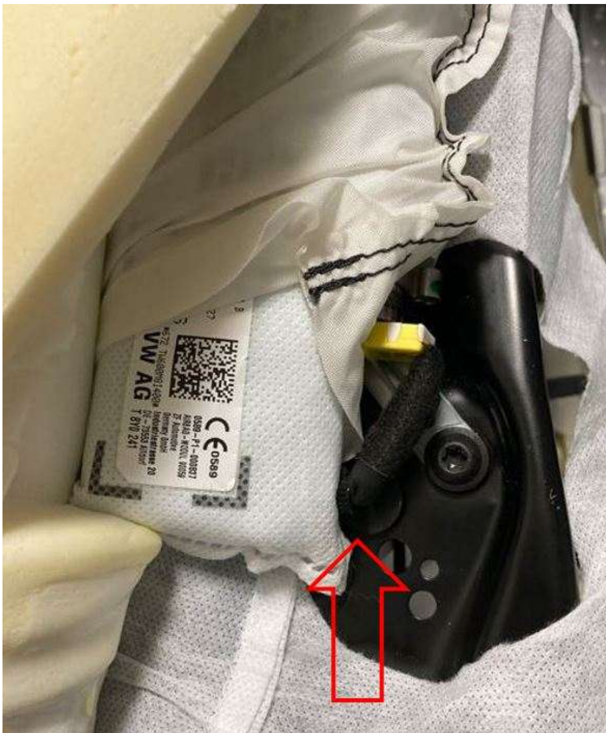
Figure 2. Attach the clip to the seat frame as shown.
