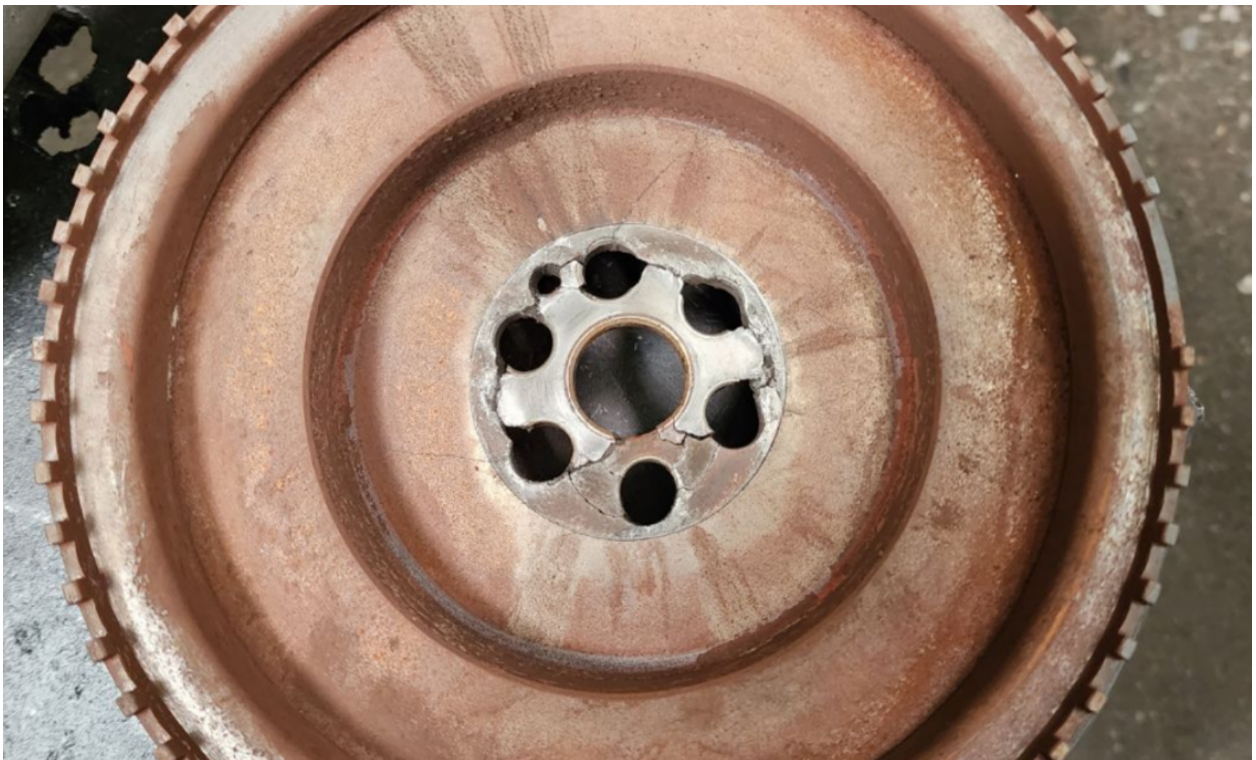
Figure 2. Example of Cracked Mounting on the Front of the Crankshaft
