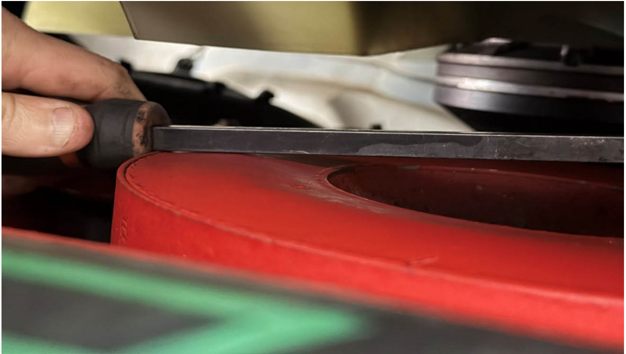
Figure 1. Example of a Swollen Engine Vibration Damper
