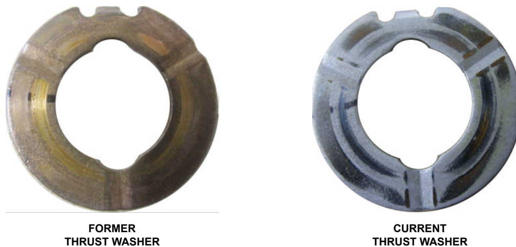
Figure 2. Example of Visual Wear Evidence of Former Thrust Washer (left) and Current Thrust Washer (right)
