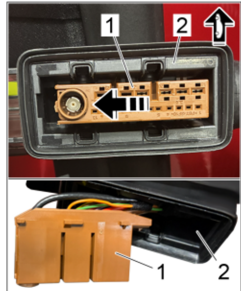
Example illustration of connector housing for door connection point
