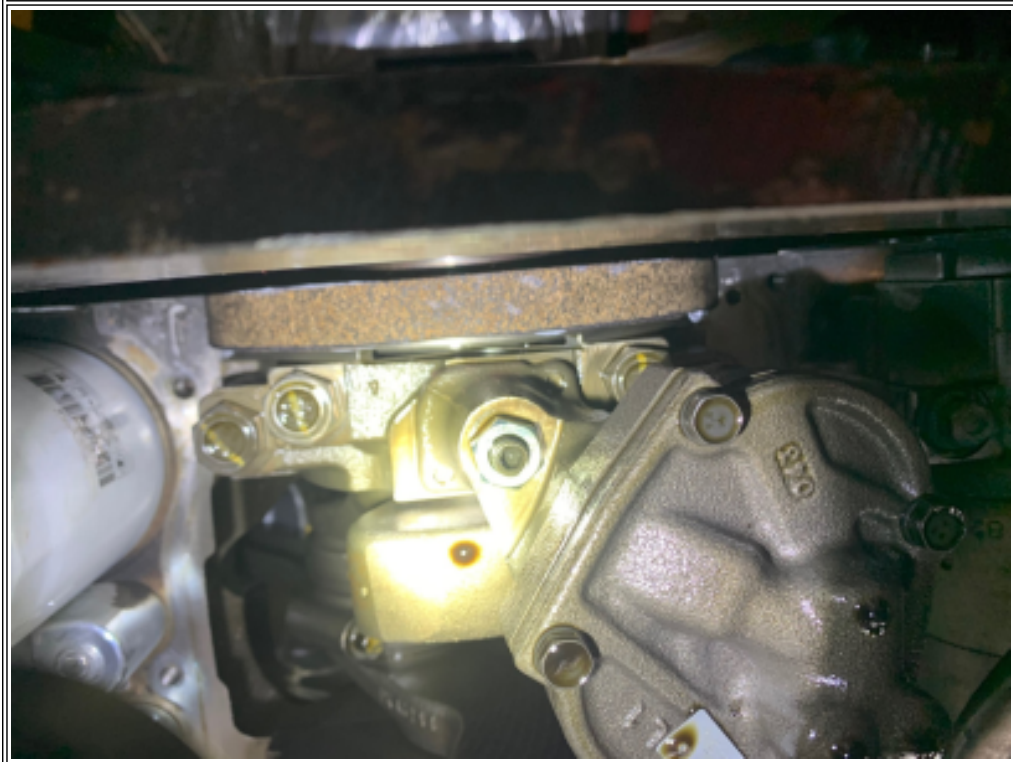
Figure 4: Cork installed with RTV on the rear main bearing cap
