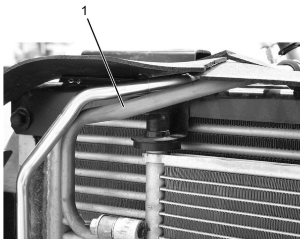
Figure 8: A/C Compressor Discharge Line - Cummins Equipped ProStar 122.
