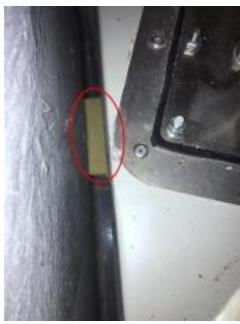
WC Area: Double-sided SM and hard styrofoam were placed between the water tank and the main body, preventing the flexibility and eliminating the noise problem. (25 minute)
