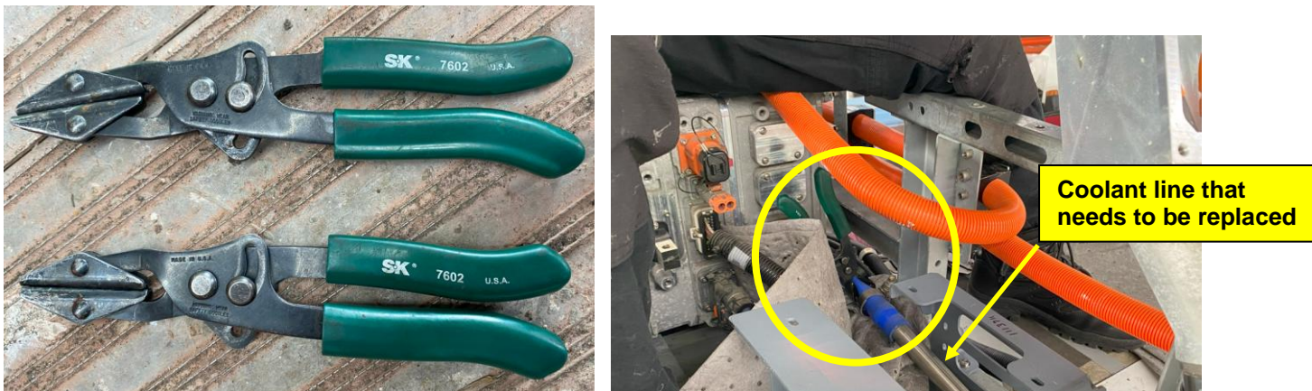
Figure 13a – Clamp coolant hoses to prevent coolant loss
