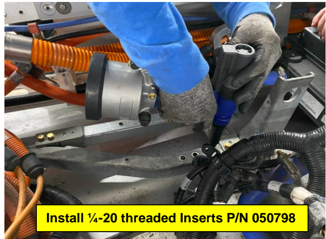
Figure 9 – Drilling holes and installing \frac{1}{4} -20 treaded inserts
