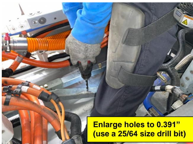
Figure 9 – Drilling holes and installing \frac{1}{4} -20 treaded inserts
