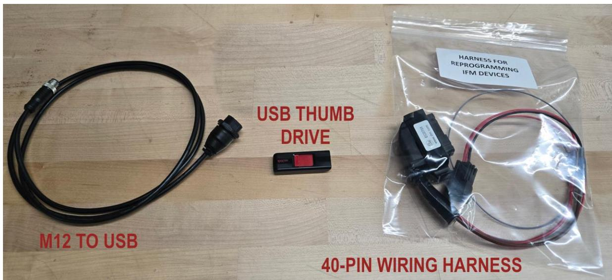
Figure 1 – Equipment Required to Reprogram Digital Instrument Cluster
