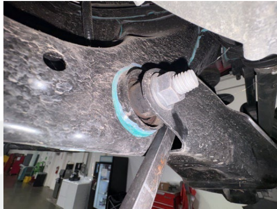
Figure 11 – Inner bushing of the LH rear lower aft link
