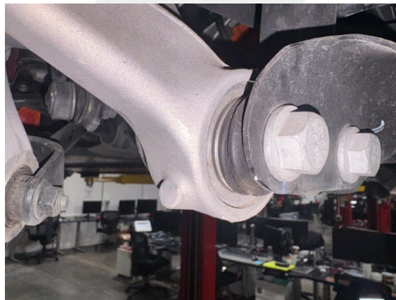
Figure 12 – Outer bushing of the LH rear lower aft link
