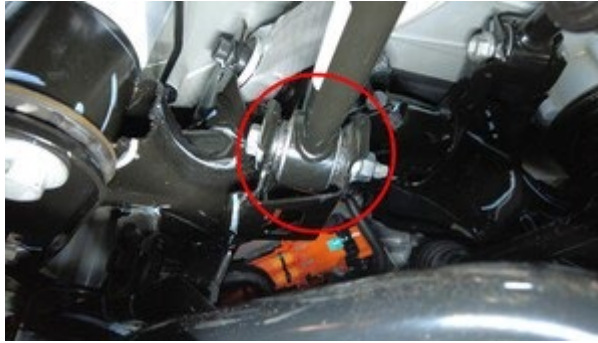
Figure 18 – Nut that attaches the LH rear toe link to the rear subframe
