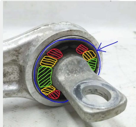
Figure 5 – RH front lower lateral link, LH similar Figure 6 – Cracking in lateral link
