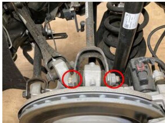
Figure 23 – Bolt that attaches the LH rear upper aft link to the rear knuckle
