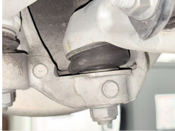
Figure 8 – LH front lower lateral link to knuckle ball joint, RH similar
