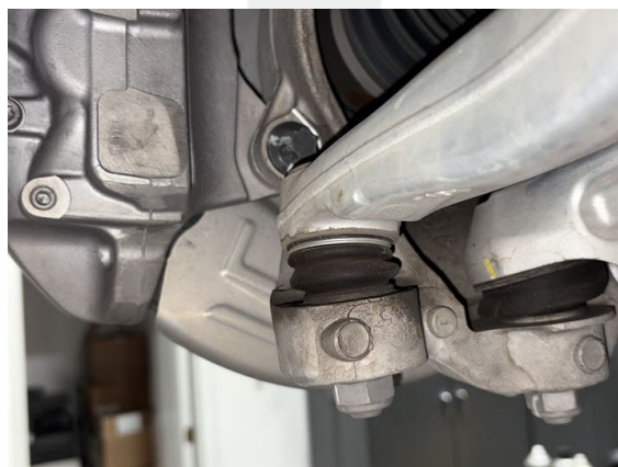
Figure 7 – LH front compliance link to knuckle ball joint, RH similar
