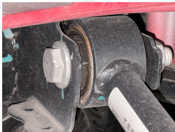
Figure 13 – Inner bushing of the LH rear upper aft link
