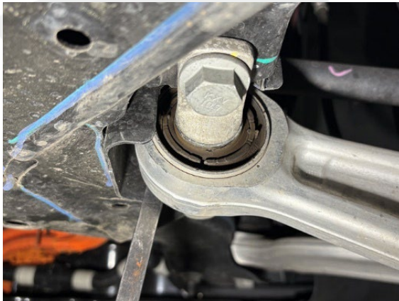
Figure 5 – RH front lower lateral link, LH similar Figure 6 – Cracking in lateral link
