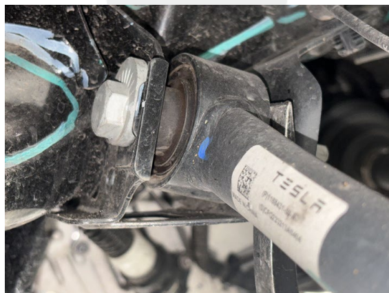
Figure 9 – Inner bushing of the LH rear toe link
