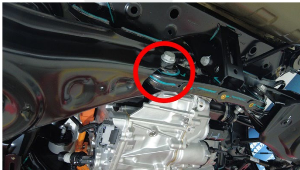
Figure 20 – Bolt that attaches the LH rear lower aft link to the rear subframe
