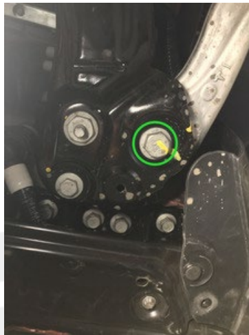
Figure 16 – Bolt that attaches the LH front lower compliance link to the subframe
