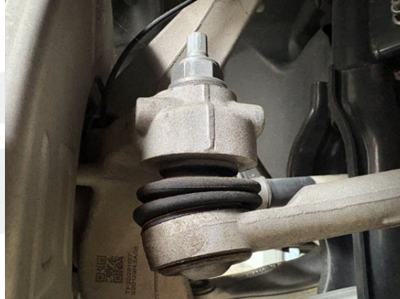
Figure 1 – RH tie rod end, LH similar
