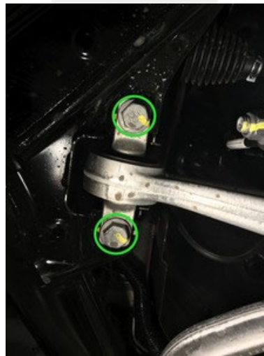
Figure 17 – Bolts that attach the LH front lower lateral link to the front subframe
