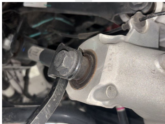
Figure 10 – Outer bushing of the LH rear toe link
