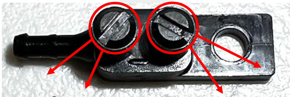
Figure 12 – Correct windshield washer nozzle cap positions and jet stream spray directions
