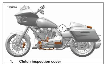
Figure 3. Clutch Inspection Cover
