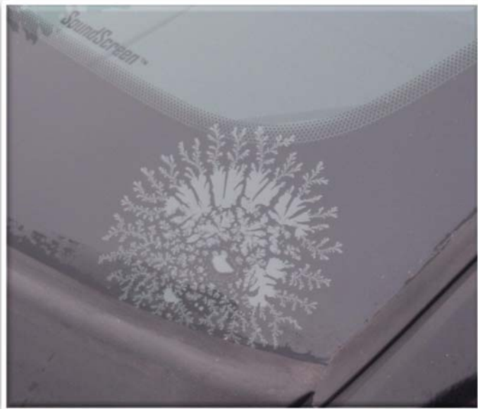
Delaminating from the glass edge Warrantable
