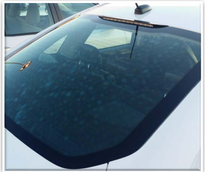
Tempered glass quench marks prominent at some angles or with polarized lenses Not warrantable
