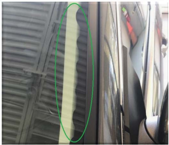
Delaminating from the glass edge Warrantable
