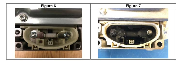
The issue shown in Figure 7 could result in no communication with the TCM, the air conditioning being inoperative, no start, or other issues. Please refer the Workshop Manual for complete information on the TCM operation and diagnostics.
