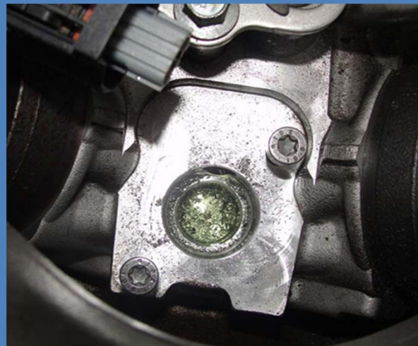
VCV port in the HP Fuel Pump
