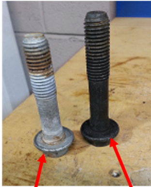
Subframe to roll restrictor bolt (shorter)
