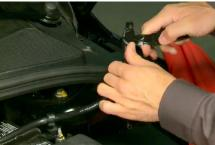
3. Remove HV service disconnect from the HV battery. Refer to Workshop Manual (WSM) for additional information.
