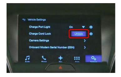
After section "a" and again after section "b" above, attempt to remove the charge cord. Wiggle charge cord handle side to side and up and down several time times, which may allow a malfunctioning cord latch to release. If this fails to work, go to stage 2.
