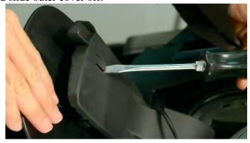
• Insert a flathead screwdriver into the slots at each of the 4 corners. Begin by gently hammering out the knock-outs in the slots. Then, using the screwdriver, pry the retaining tabs away from the sheet metal and pull the charge port housing out at each corner.
