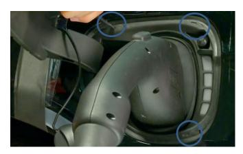
5. Locate the manual lock release lever inside charge port opening as shown. Using the flathead screwdriver, access the manual lock release lever and pull the lever towards the outside of the vehicle.
