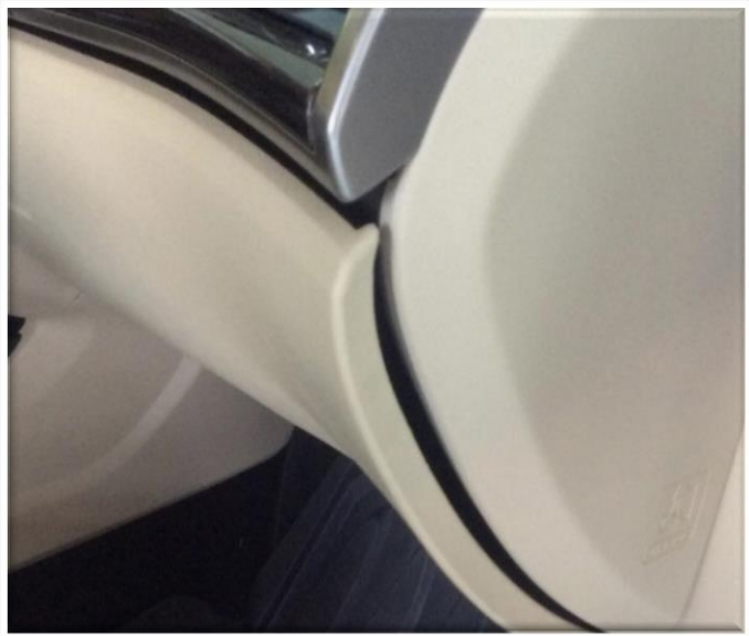
Gaps that cannot be corrected with adjustment.
