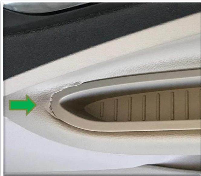
Loose material/trim that cannot be adjusted. Warrantable
