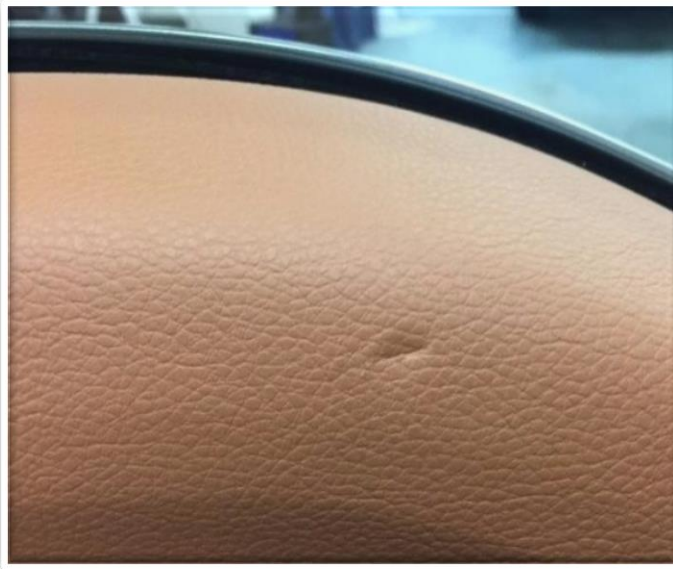
Scratches, indentations or cuts which intersect the grain pattern of the material. Not warrantable
