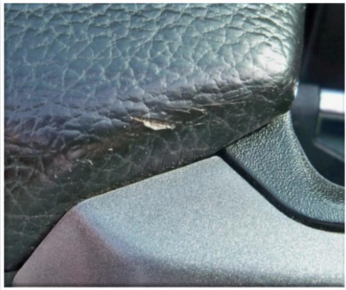
Scratches, indentations or cuts which intersect the grain pattern of the material. Not warrantable
