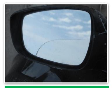
A single crack (without impact refer to Pen Test below), either curved or straight with no splintering, is due to mirror imperfections and thermal stress from mirror heat. Replacement of mirror assembly may not be required, service lowest level possible (glass sub-assembly). <u>Warrantable</u>
