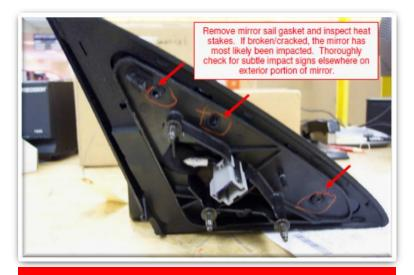
Heat stakes broken / cracked is an indication that the mirror may have been impacted <u>Not warrantable</u>
