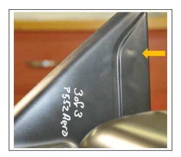
Bubbles or blistering without surface grain distortion, surface melting or warping may be an indication of air entrapment or tempature varation during the molding process. <u>Warrantable</u>
