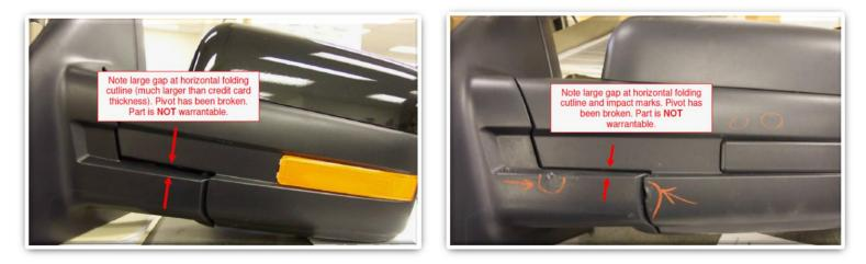
Broken pivot is an indication that the mirror may have been impacted. Thoroughly inspect the mirror for subtle impact signs and measure the gap at the folding cutline. Large gap in the cut line with or without impact marks on the mirror is: <u>Not warrantable</u>
