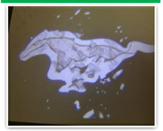
Moisture is apparent in lamp. Replacement of mirror assembly may not be required, service lowest level possible (courtesy lamp). Warrantable
