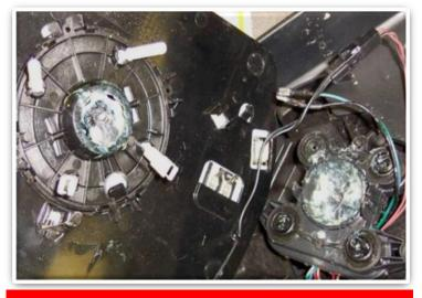
Actuator is broken due to disassembly of mirror glass outside of WSM procedure or from impact damage Not warrantable
