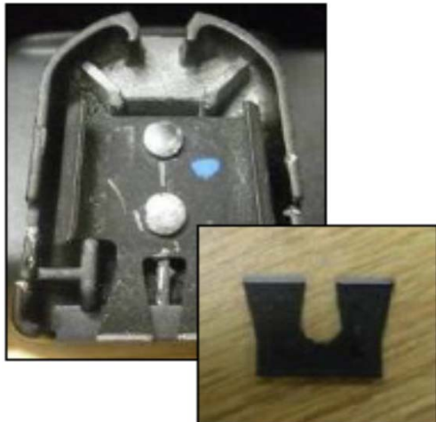
Improper removal can cause the clip to break. These are definitive signs of improper removal and therefore NOT warrantable.
