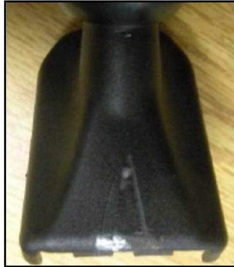
Scratch marks on the outside of the show improper removal.
