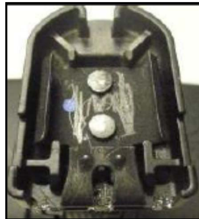
Scratch marks on the inside of the mount indicate that the mirror was removed incorrectly. These are definitive signs of improper removal and therefore NOT warrantable.
