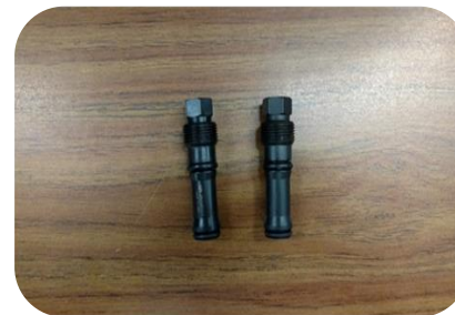
High Pressure Stand Pipe Block Off Plugs 303-1071 - Build Date: 9/30/03 - 7/18/04
