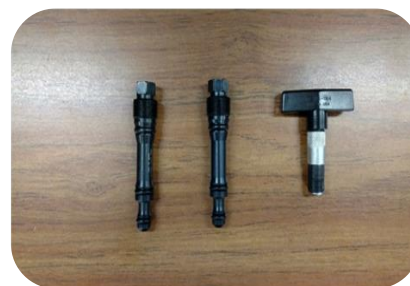
High Pressure Stand Pipe Block Off Plugs 303-1163 and Stand Pipe Removal Tool - Build Date 7/19/04 and up
