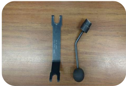
Disconnect tool quick release coupling 03-755 and injector plug release tool
