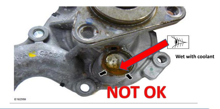
Coolant pump will have wet coolant residue with an evident puddle occurring on the pump weep chamber.
