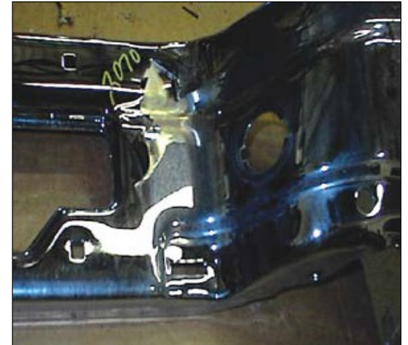
Aftermarket Remanufactured / Rechromed Bumpers with Poor Replate and Ford oval partially removed
