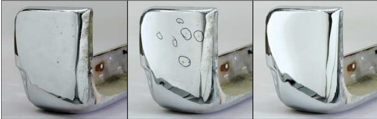
Chrome Bumper – Lack of Maintenance (before / after cleaning)
