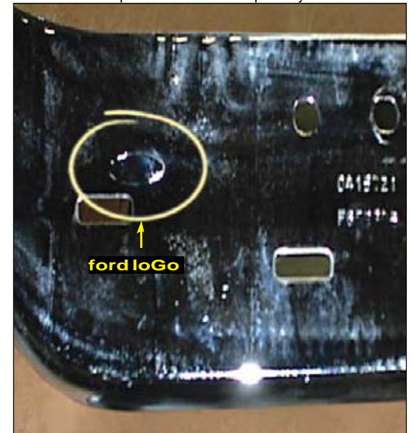
Aftermarket Remanufactured / Rechromed Bumpers with Poor Replate and Ford oval partially removed
