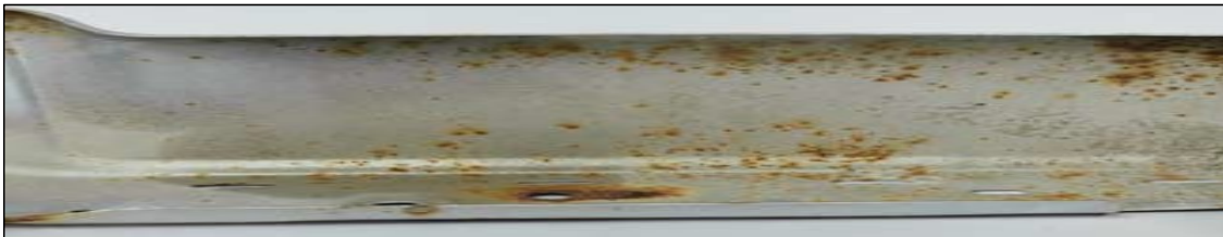
Chrome Bumper – Corrosion on Backside of Bumper
