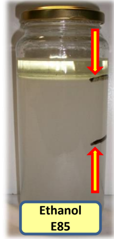
Figure 3 – Ethanol E85 added then shaken. Note the large increase in the water level.
