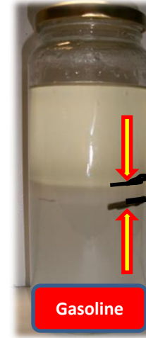
Figure 2 – Gasoline added then shaken. Note the small increase in the water level.
