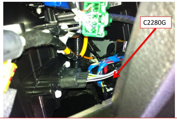
C2280G Is located on the right hand side of the vehicle, behind the glovebox
