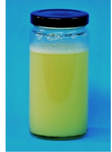
Figure 6 – Water emulsified in fuel
