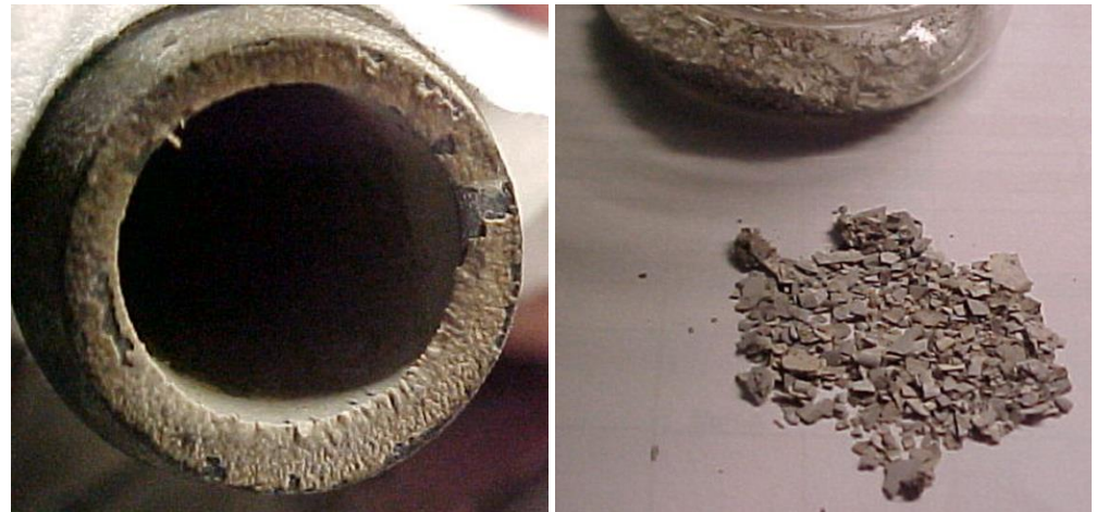
Figure 2. Scale buildup inside oil cooler
