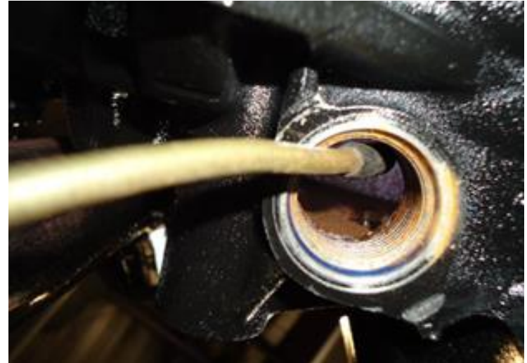
Figure 3: Inspection through block drain using flexible borescope.
