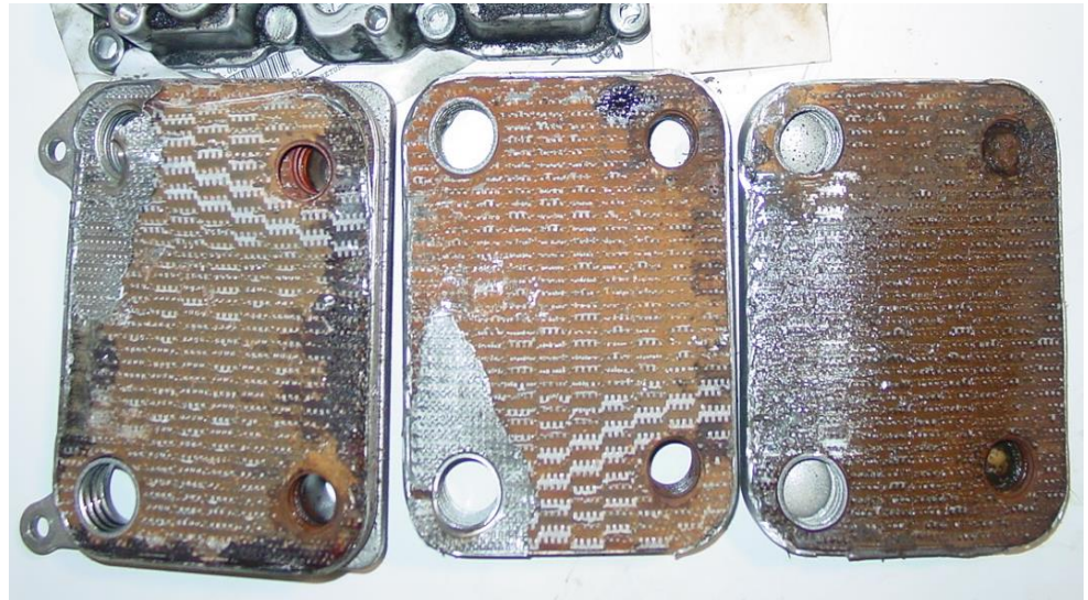
Figure 1. Restricted internal oil cooler passages
