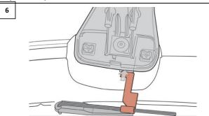
Using the supplied torque wrench, insert the red tab into the slot as shown. Slide tool in until it makes contact with the Lon the casting
