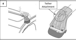
Attach the tethers from stanchion to cover. Lower the end cap covers onto the crossbar and slide outward to engage the tangs. Rotate downwards to fully snap cover into position.
