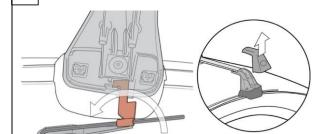
Rotate the tool using the Allen wrench as a handle to push the back of the tool against the L and the "hook" against the cover tab until the tab pops loose.
