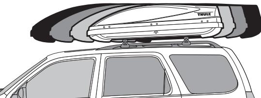
**NOTE:** Mount box towards the rear of the vehicle to minimize wind resistance.
