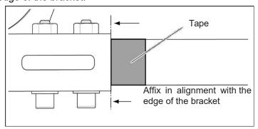
(3) Draw a positioning line on the tape at the extended position of the alignment marks on the bracket.
