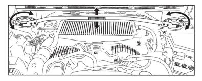
(10) Tighten the flange nuts to the specified torque. Tighten the two nuts that are closer to the back of the vehicle first and then the one nut that's closer to the front of the vehicle.
