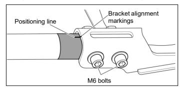
(3) Remove the M6 bolts (total of four on left and right) connecting the bar to the brackets and then remove the brackets.
