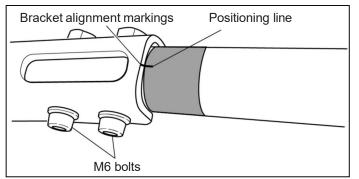
(4) Remove the two M6 bolts connecting the bar and the bracket on the right side of the vehicle and then remove the bracket on the right side of the vehicle.
