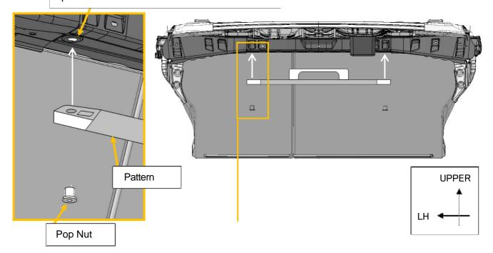
Once the position is determined, secure the rear bulkhead, pattern and pop nut with tape.
