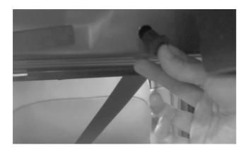
2) Insert the bolts into the 2 holes on the underside of the guard bar and temporarily assemble them with the pop nuts.
