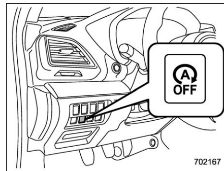
Auto Start Stop OFF switch
