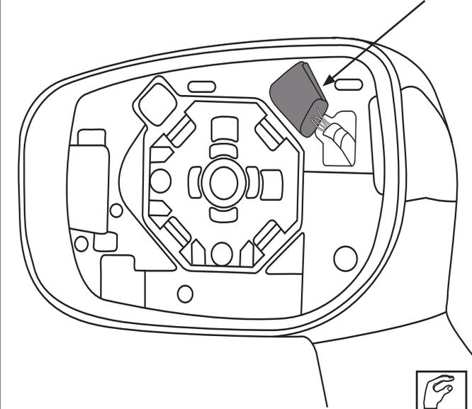
Locate and remove prearranged vehicle connector. (a)
