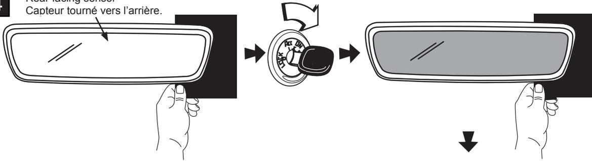
To test the dimming function, cover the forward facing sensor and shine light on the interior mirrors rear facing sensor.
