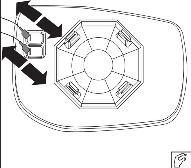
If equipped, disconnect heater terminals.
