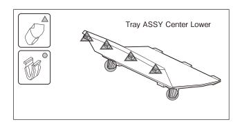
(3) Open the Console Lid, pull up the Cover ASSY Front, and disengage the clips (18 places).
