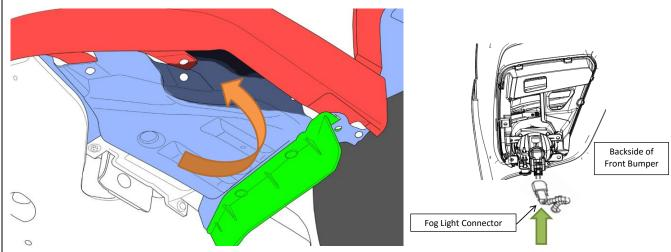
STEP 24: Re-install 3 clips and the inner wheel well clip on each side.
