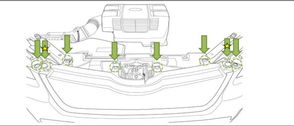
STEP 23: Reconnect fog light connector on both sides. Skip to Step 24 for vehicles without fog lights.
