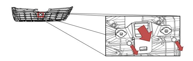
STEP 12: Unpack new sport grille onto a soft surface. Reuse the 2 screws from the previous step and install the new cover bracket onto the sport grille. Be sure to use the rectangular guidance hole to help with installing new cover bracket. Torque screws to 13 in-lbs ± 4 in-lbs (1.5 N·m ± 0.5 N·m).
