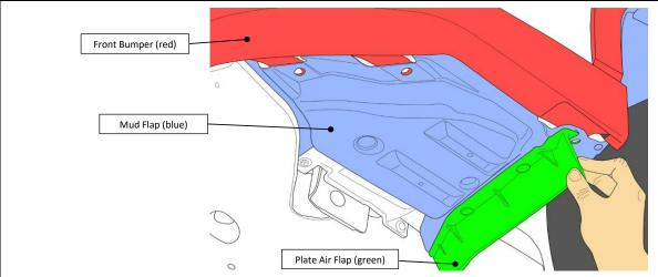
STEP 6: For vehicles with fog lights, fold mudguard inward, reach in, disconnect fog light connector. Repeat on other side. For vehicles without fog lights, skip to Step 7.
