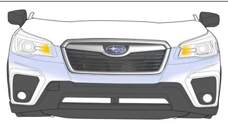
STEP 3: Tape both headlights and fenders, hood latch lever and areas around the grille as shown.
