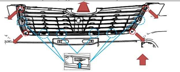
STEP 11: Place original grille on soft surface. Remove the 2 screws from the back of the grille and discard original cover bracket.
