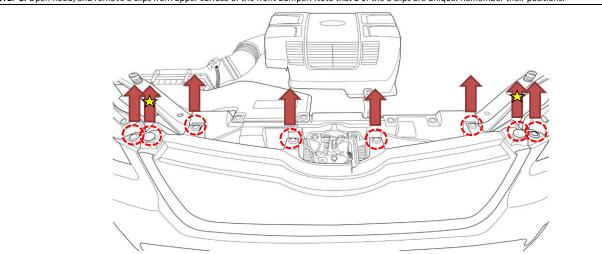
STEP 9: Note the location of the tabs in the image on the left. Carefully start removing the front bumper by pulling outward from the sides and then forward. Disengage each tab carefully and slowly. Excessive force can break a tab. Fully remove front bumper and gently place on a soft surface.
