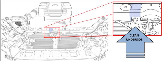
**STEP 18**: Attach the foam cushion so that the sticky sides attach to the underside of the vehicle's frame. Pay attention to the diagram that shows the front of the vehicle in relation to the sticky sides of the foam cushion. Press down firmly to bond both surfaces.
