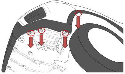
STEP 5: Take a picture or study how the front bumper, mud flap, plate air flap assemble together. Note the overlap sequence.
