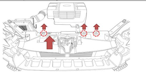
STEP 17: Use isopropyl alcohol to clean UNDER the area indicated in the image below.
