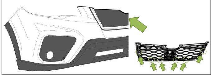
STEP 14: Re-install the 4 screws to secure the sport grille to the front bumper. Torque all screws to 13 in-lbs ± 4 in-lbs (1.5 N·m ± 0.5 N·m). Set aside front bumper with sport grille on a soft surface.
