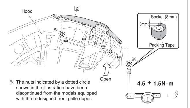
Do not allow any of the nuts to drop into the engine compartment.
