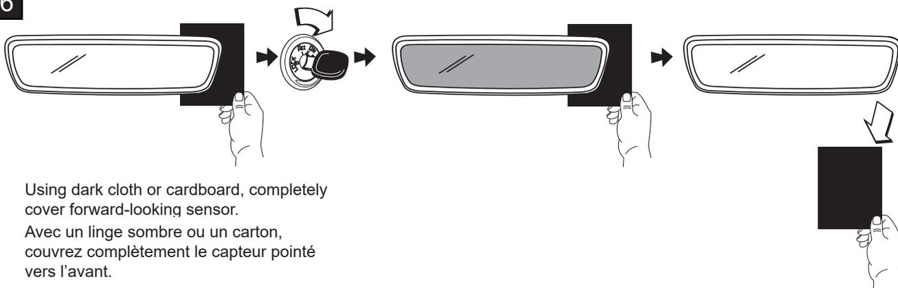
Using dark cloth or cardboard, completely cover forward-looking sensor.
