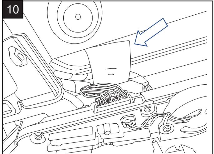
1. Plug jumper harness into pre-wire connector and mirror and
