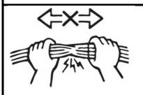
Be careful not to forcefully pull the wiring harness of the vehicle. This helps prevent the connector from being disconnected, and the wires from being cut or damaged.
