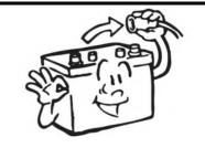
Please disconnect the negative battery cable while conducting wiring operations. Failure to do so may result in electric shock or injury.
