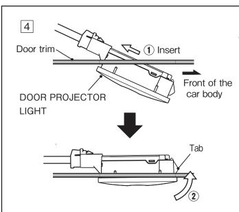
Insert the DOOR PROJECTOR LIGHT into the door trim. Ensure the front side tab is locked at the correct position.
