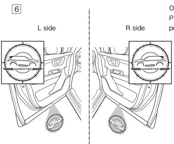
Open the door and confirm the DOOR PROJECTOR LIGHT's image is correctly projected.
