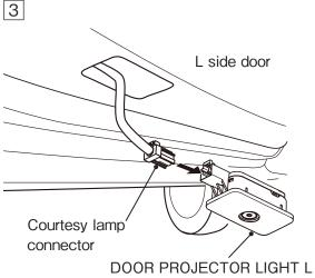
Confirm L/R side is correct. Connect the DOOR PROJECTOR LIGHT to the courtesy lamp connector.
