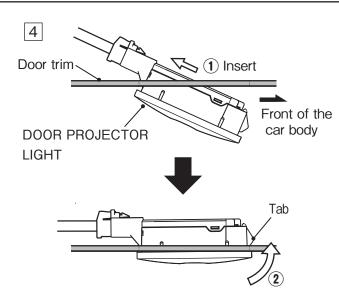
Insert the DOOR PROJECTOR LIGHT into the door trim. Ensure the front side tab is locked at the correct position.
