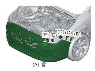
While pushing up the lower side (A) of the bumper face front, release the engagement in the order from (B) to (F).
