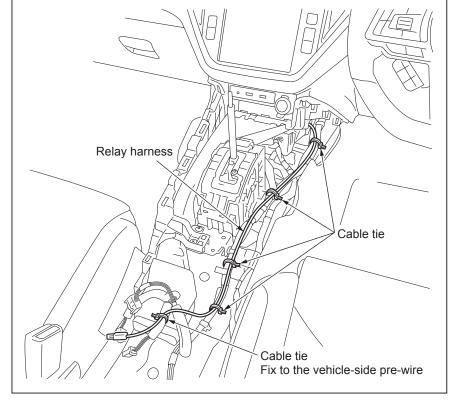
(4) Connect the connectors of the relay harness and vehicle-side pre-wire to the CD PLAYER cable connectors.
