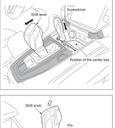
(1) Turn over the rubber of the center tray, insert the screwdriver into the position in the figure, and while inserting it to the depth, lower the shift lever.
