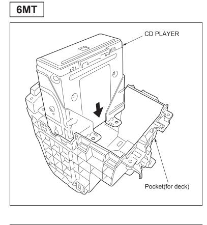
(8) Install the CD PLAYER while passing the CD PLAYER cable through the hole in the pocket (for deck).
