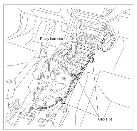
(2) Wire the relay harness along the vehicle harness, and fix it with a cable tie.
