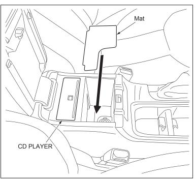
(8) After reinstalling the vehicle components, attach the mat in the console box ASSY.
