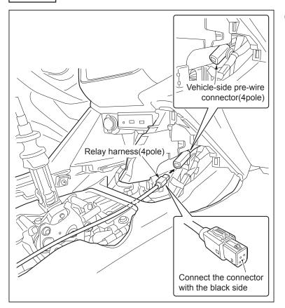
Connect the connector with the black connection side of the relay harness to the vehicle-side pre-wire connector.
