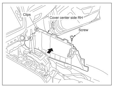
(7) Remove the screw, and then remove the cover center side RH.(Clips: 2 points)
