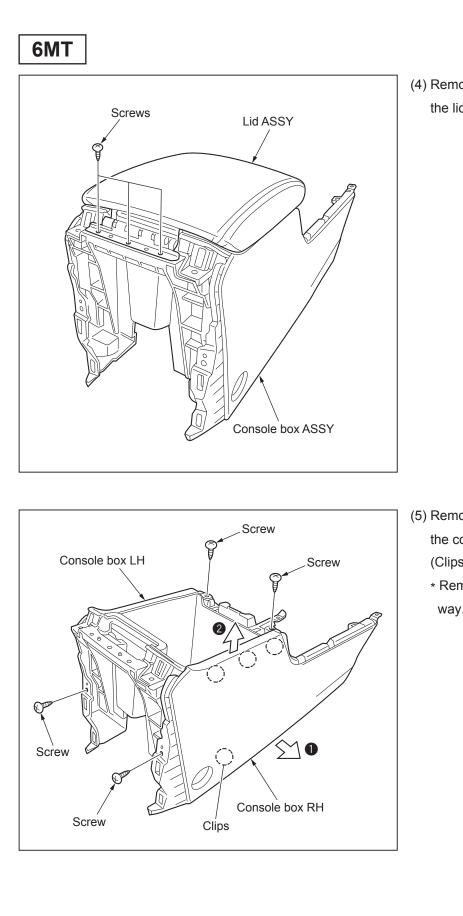
(4) Remove the three screws, and then remove the lid ASSY.
