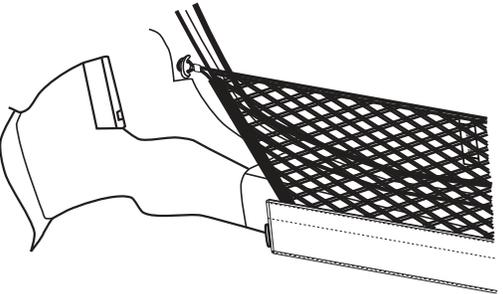
(b) Place each bungee loop around the upper T-anchor as shown in graphic.
