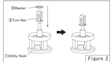
3. Turn the utility hook ① clockwise by hand to install it to the rear gate.
